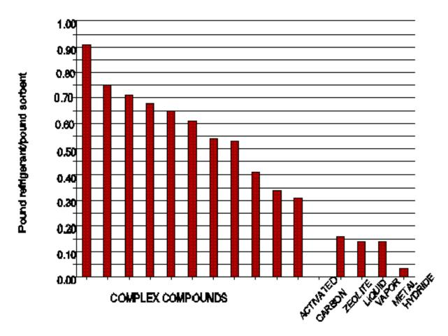
*Figure 2 Refrigerant holding capacity of complex compounds compared to other sorption media.*
